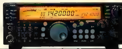
TS-570D HF base station
